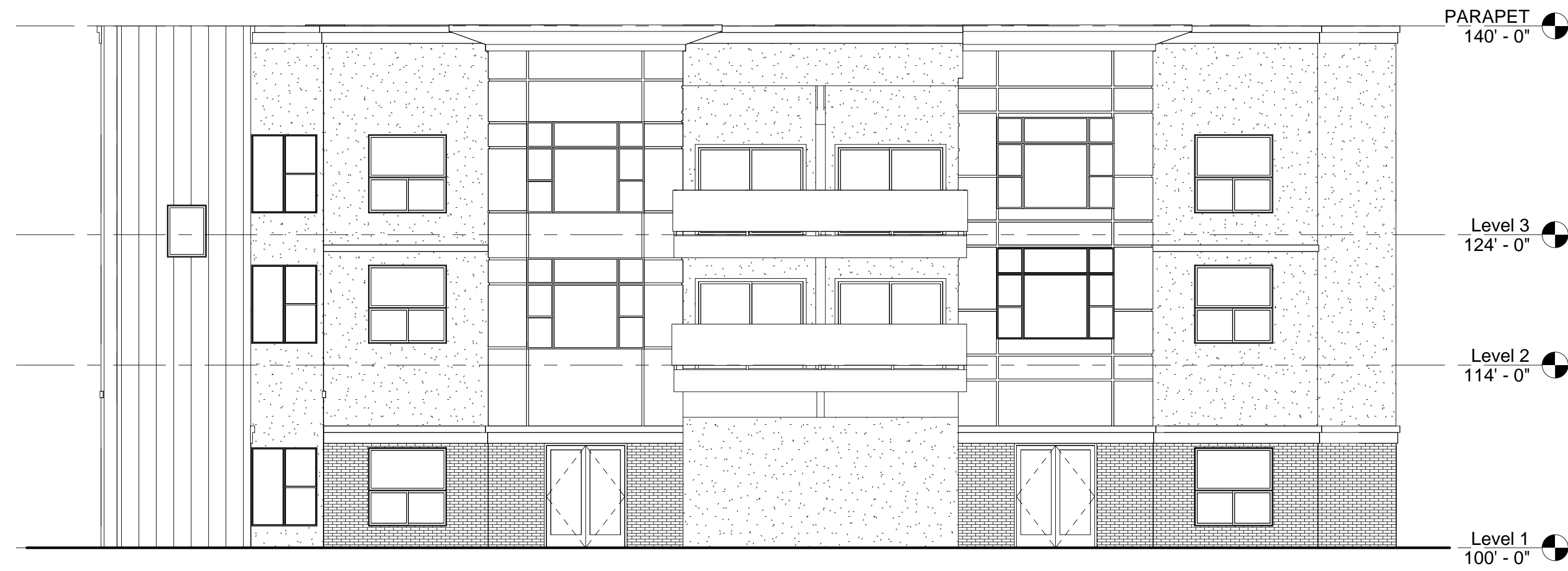
WEST ELEVATION SCALE 1/8" = 1'-0"
